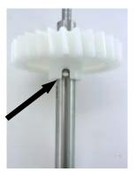
Step 2: Insert the worm gear driven from the bottom so that the pin slides into the slot.
