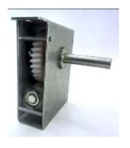
Step 12: Insert the worm pinion assembly into the end plate through the side that has the bearing flanged out.
