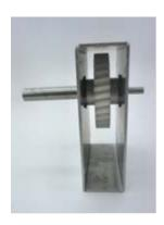
Step 11: Press in a ##bearing## to the end plate.
