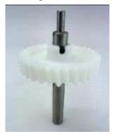
Step 4: Slide in the two metal spacers onto each side of the worm gear driven.
